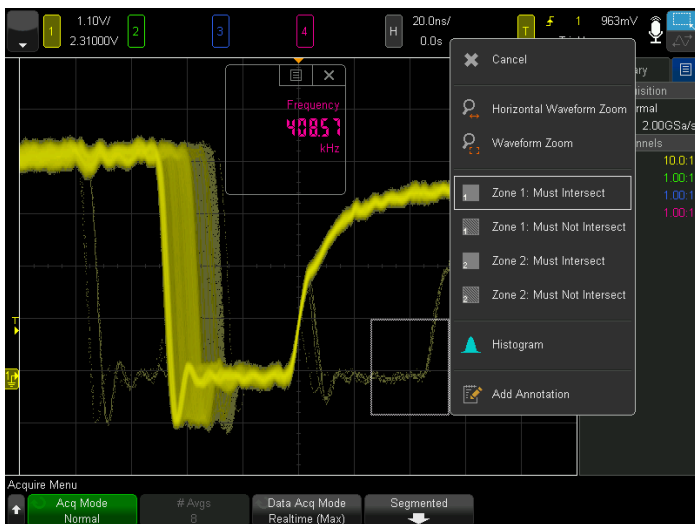
Figure 11. Draw a zone (box) around the anomaly.
