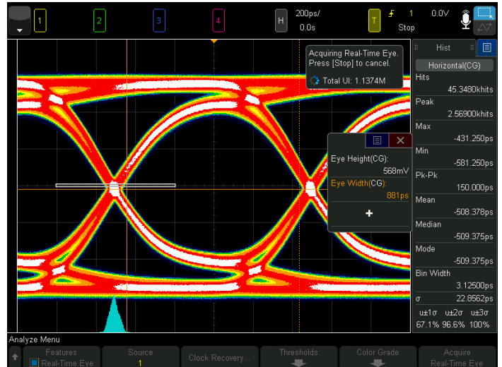
Figure 20. A real-time eye diagram measurement of a clean 1-Gbps PRBS embedded clock signal. The histogram measured about 22-ps rms jitter.
