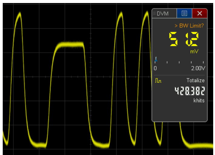
Figure 35. Totalizing the number of runt errors.
