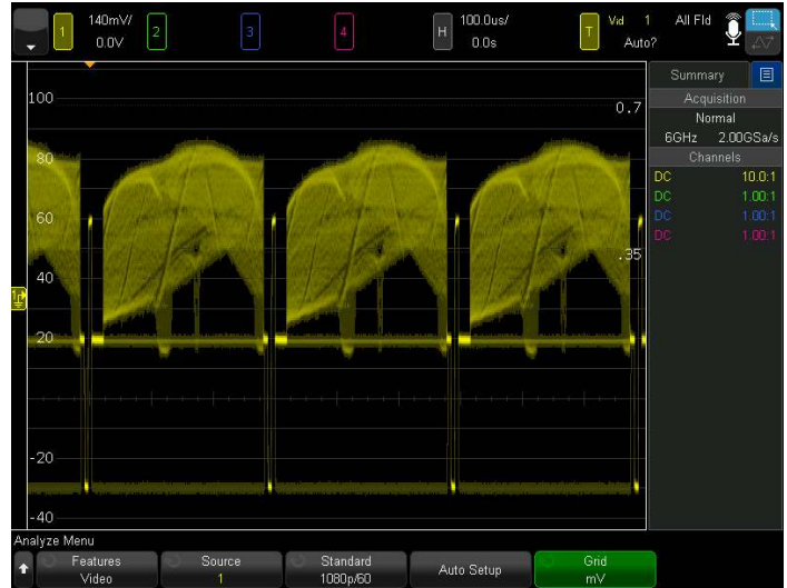
Figure 45. Triggering on a 1080p/60 signal.
